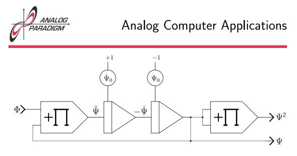
Figure 1: Setup for the one-dimensional SCHRÖDINGER equation
